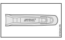
Your saw comes standard with a chain scabbard that matches the cutting attachment.
