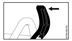
Pull the hand guarad towards the front handle until there is an audible click – the chain brake is disengaged.
