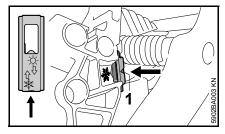
Place the shutter with the opening in the direction of the chain saw (winter operation) – arrow points toward symbol \* – shutter must audibly snap into place
