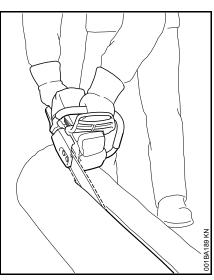
Cutting technique in which the spiked bumper is not used – risk of pull-in – start the cut with the guide bar at the shallowest possible angle – take extra care since there is an increased **danger of kickback**.
