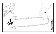
Retensioning during cutting work:
