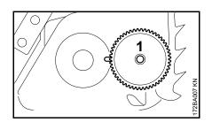
Fitting the tensioning gear
