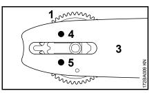
Position the tensioning gear (1) against the guide bar (3) so that the stud (4) projects through the upper hole and the short guide peg (5) locates in the lower hole.
