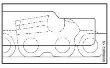
Lay the file gauge on the saw chain
