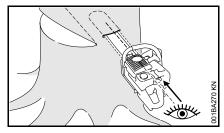
Where possible, use a plunge blade. The plunge blade and the upper/lower side of the guide bar are parallel.
