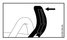
Pull the hand guarad towards the front handle until there is an audible click – the chain brake is disengaged.
