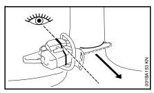
Insert the chainsaw with guide bar in the bottom of the felling notch. The gunning sight must point in the planned direction of fall – if necessary, correct direction of fall by re-cutting the felling notch.
