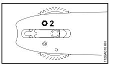
• Screw the nut (2) on to the stud as far as stop by hand.
