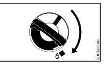
While holding the cap depressed, turn it clockwise until it engages in position.
