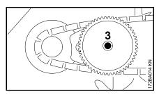
Fit the chain sprocket cover so that the wingnut locates on the collar screw (3).
