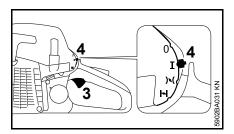
Press the throttle trigger lockout and blip the throttle trigger (3); the master control lever (4) jumps to run I and the engine begins to idle
