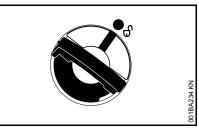
Marks on tank cap and fuel tank must line up.
