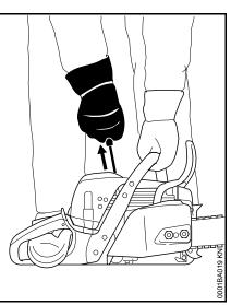
With the right hand, pull the starter grip slowly until you feel it engage – and then give it a brisk strong pull – simultaneously press down on the handlebar – do not pull the starter rope out all the way – risk of breakage! Do not let the starter grip snap back – guide it vertically back into the housing so that the starter rope can rewind properly
