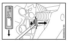
Using the combination wrench or a screwdriver, pry the shutter out of the
