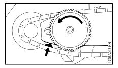
Make sure the drive link tangs engage the bar groove (see arrow) and then rotate the tensioning gear counterclockwise as far as stop.
