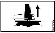
• Remove the tank cap.
