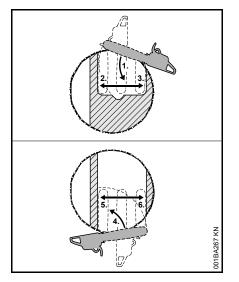
Perform this felling cut when the tree diameter is greater than the cutting length of the chainsaw.
