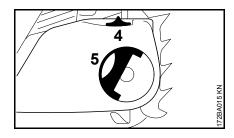
When fitting the chain sprocket cover, check that the teeth of the tensioning gear and adjusting wheel mesh properly.
