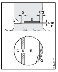
The **felling notch** (C) determines the direction of fall.
