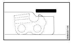
Rework the depth gauge so that it is flush with the file gauge
