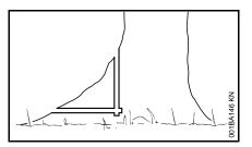
Remove largest buttresses: first the largest buttress – saw first vertically, then horizontally – only if the tree is in sound condition
